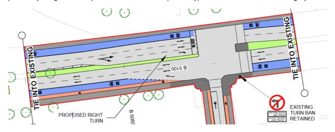
Image 4.22: The Preliminary Design of the Proposed Scheme at the Chapelizod Bypass which Ties in with the Existing Layout
