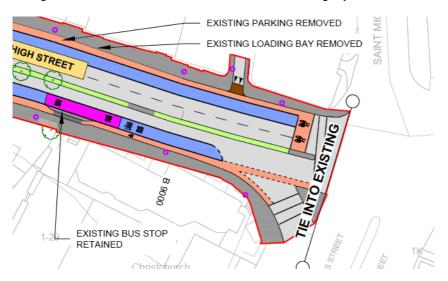
Image 4.26: The Preliminary Design of the Proposed Scheme at the Junction of High Street and Winetavern Street with the Existing Layout
